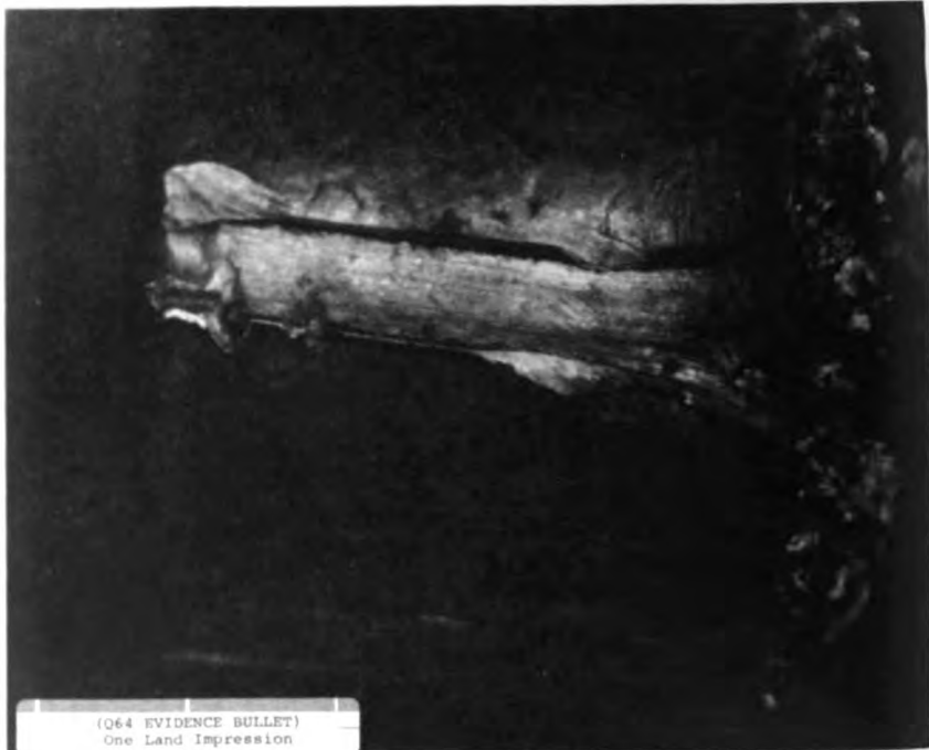
FIGURE 10. —Photomicrograph of one of the land impressions on the Q64 bullet removed from Dr. King's body. It shows the type of damage sustained by the bullet.
