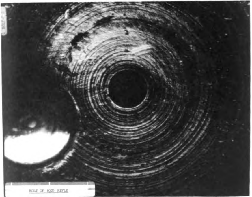
FIGURE 12.—Photomicrograph showing the individual identifying characteristics (machine marks) on the bolt face and the location of the ejector of the Q2 rifle.
